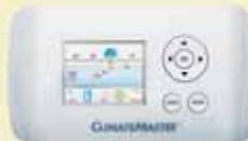
What is truly revolutionary about the iGate® Connect system is that dealers (from their office, home or vacation) can now monitor unit operation (47 data points), faults (including details and conditions at fault) and change settings (15 settings) from an internet-connected computer or mobile device.
