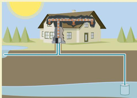
Open-loop installations actually pump water from an underground aquifer through the geothermal unit and then discharge that water to a drainage ditch or pond. The geothermal unit processes the heat energy from the water just like a closed-loop installation. Discharging water to a "return" well is sometimes effective, but sending water to a pond or lake is considered more reliable.
